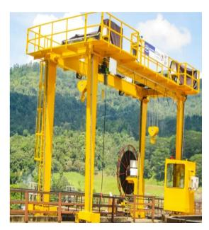
This type of cranes is used in the area where the building was not designed to bear the crane load and the outdoor applications where there is no building coverage.
